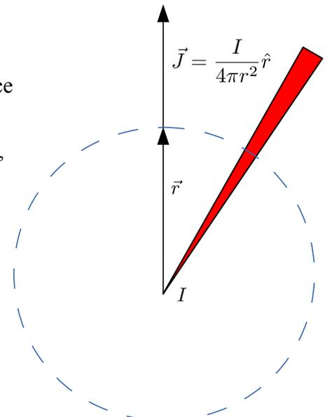
Figure 2. Current  $I$  injected at the origin of the system spreads uniformly in all directions in infinite, homogeneous and isotropic medium.
